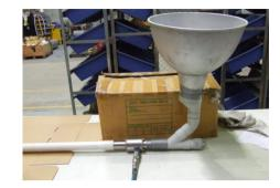
Also tried 5 metres rising up to 1800mm, through 90 degree elbow down into drum. 56 Seconds.
