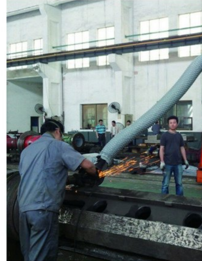
Fume extraction for the metal piece cutting
