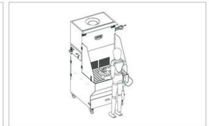
Small work piece welding fume extraction
