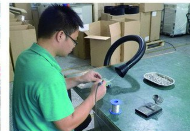
PCB soldering fume extraction
