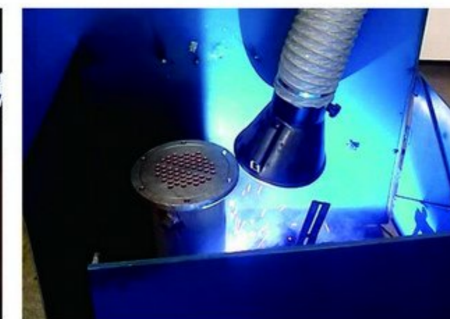
welding workshop supported fume extraction
