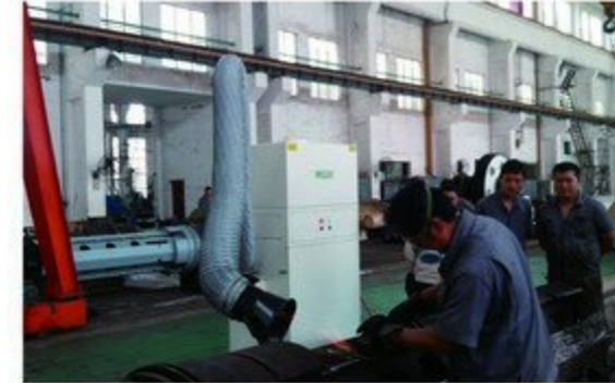
Steel pipe grinding supporting dust cleaning
