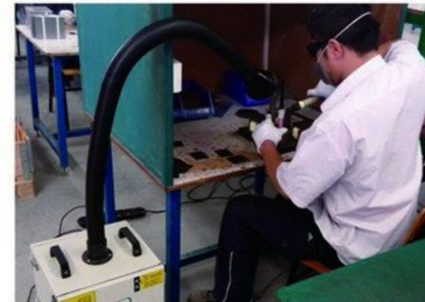
small-sized transformer welding supported fume extractor
