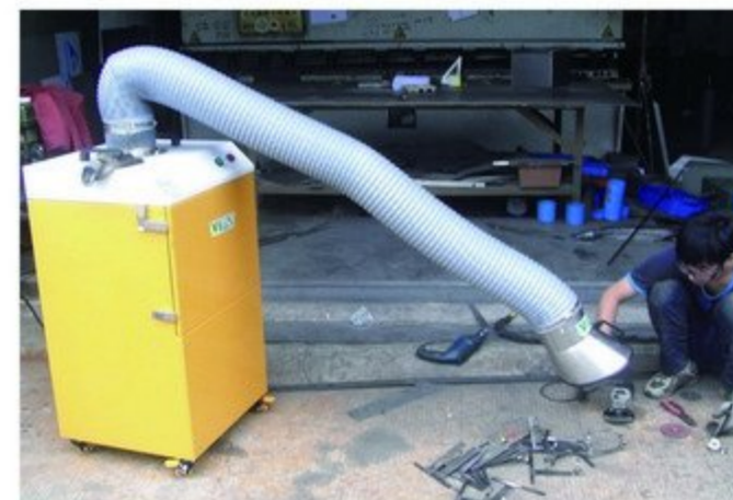
Sheet metal processing workshop supported fume extraction
