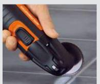
If tile joints need to be removed completely and renewed, the round diamond saw blade is the most costeffective solution – both in terms of work progress and service life.
