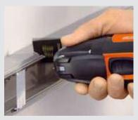
The E-Cut standard saw blade is ideal for cutting plastic construction elements such as cable ducts, exhaust air pipes or downpipes.
