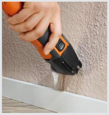
The M-CUT saw blades can be used to make very fine cut-outs and recesses. The saw blades are suited to virtually all materials such as wood, hard wood, plastics, fibreglass and sheet metals up to 1 mm.
