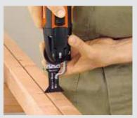
The depth stop can be used to set the cutting depth of all E-Cut saw blades and the HSS saw blade for wood in a continuously variable manner.
