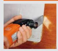
The M-CUT saw blade proves itself when subsequently installing electrical or electronic devices. For clean sawing edges without damaging high-quality materials.
