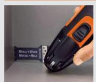
The E-CUT saw blades can be used to make space for cable entries, sockets and water connections in cupboards and shelf units without the need for laborious dismantling.
