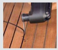
The cutter blades can be used to thoroughly remove deck joint materials at speed. The working time for this application is cut by 80%. More time is saved when satin-finishing teak decks.
