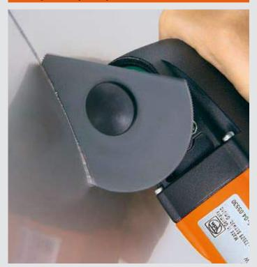
Sheet metals and plastics up to approx. 1 mm thick can be cut burrand warp-free using the HSS segment saw blades. This results in minimum sparking and avoids laborious rework. They can also be used universally in corner areas.
