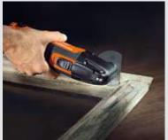
The HSS segment saw blade can be used to perfectly renovate old windows and allows you to work fatigue-free right into corners without the need for time-consuming rework.
