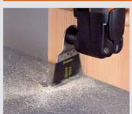
The E-Cut saw blades can easily saw recesses for subsequent installations and conversions, even if worktops have already been fitted.
