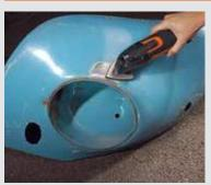
The FEIN MULTIMASTER is made for applications such as paint errors, defects and areas that would normally be sanded by hand. A high sanding capacity and even sanding pattern are guaranteed.
