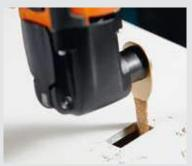
Recesses and openings can be deburred and filed to perfection with the carbide file.
