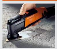
Using the carbide rasp to sand down plaster, cement, concrete or tile adhesive eliminates the need for time-consuming and laborious manual work.
