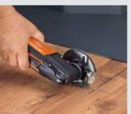
When used in conjunction with the depth stop, the HSS saw blade for wood is ideal for making subsequent cut-outs in laid parquet or laminate flooring.
