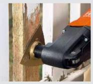
The carbide rasp can be used to thoroughly remove even the most stubborn signs of weathering at speed thanks to the high sanding capacity.
