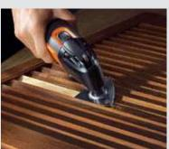
The flat sanding pad allows you to reach into even tight gaps such as the slats of window shutters.
