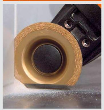
The segment saw blade is used to remove damaged tile joints in corners and on edges, as it enables precise working without overcutting. The segment saw blade is available in carbide or diamond quality. Diamond saw blades offer impressively longer service lives and are also suited to frost-proof joint materials containing epoxy resin used outdoors or to replacing joints.
