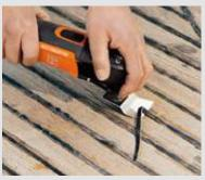
The rigid stopper knife can be used to cut back excess polyurethane joint materials after jointing at speed and with precision. This saves a lot of time and effort later when it comes to sanding down the teak deck.
