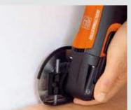
The HSS saw blade for wood transforms the FEIN MULTIMASTER into a "mini circular saw" which is ideal for long, precise cuts such as expansion joints in parquet and laminate. Can be used with or without depth stop. Order number 3 26 07 065 02 0
