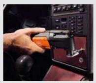
The MINICUT and file set can handle tiny cuts from 10 mm with ease – even if they're in hard-to-reach places. Can be used for plastics, metals and wood.
