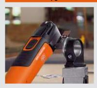
The FEIN MULTIMASTER can be securely clamped into all standard drill jigs using the table and drill jig holder – for extremely precise results. Alternatively, you can also attach the FEIN MULTIMASTER directly to the workbench or work table. This keeps your hands free to guide the workpiece safely.
