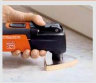
Natural or plastic window sills can be optimally machined with the special range of sanding materials and the felt polishing pad.
