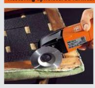
The stepped HSS saw blade saves your effort and upholstery, as staples can be removed with ease and do not have to be pulled out with pliers.
