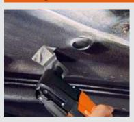
The rigid stopper knife can also be used to remove underseal and other stubborn coverings in the best possible time.
