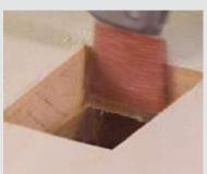
Recesses can be filed with precision using the MINICUT and file set.
