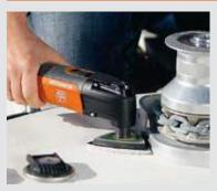
Using the bristle fleece in conjunction with yacht cleaner ensures that fibreglass surfaces with anti-slip structures are cleaned thoroughly.
