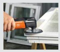
The round backing pad enables accurate sanding on edges and folds without kick-back.
